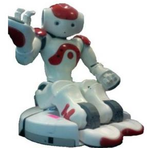
Nao robot mounted on an iCreate platform
